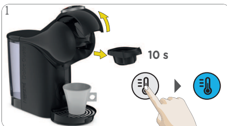
Open the locking handle. The machine switches on automatically. Press the temperature selection button within 10 seconds after starting the machine to change to cold mode (blue). A cold beverage can be prepared immediately.
